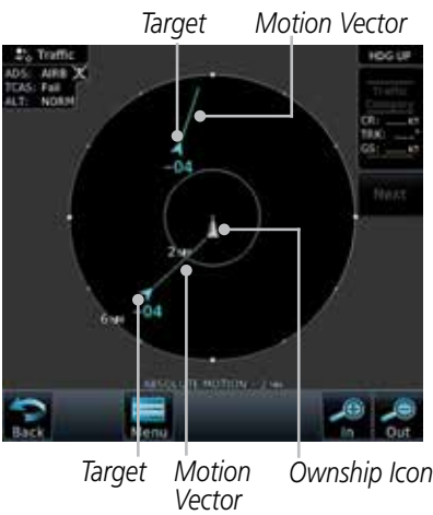
Figure 10-16 Comparison of Absolute and Relative Motion Vectors With a Two Targets
