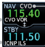
Figure 3-27 Automatic Nav Frequency Ident Decoding
