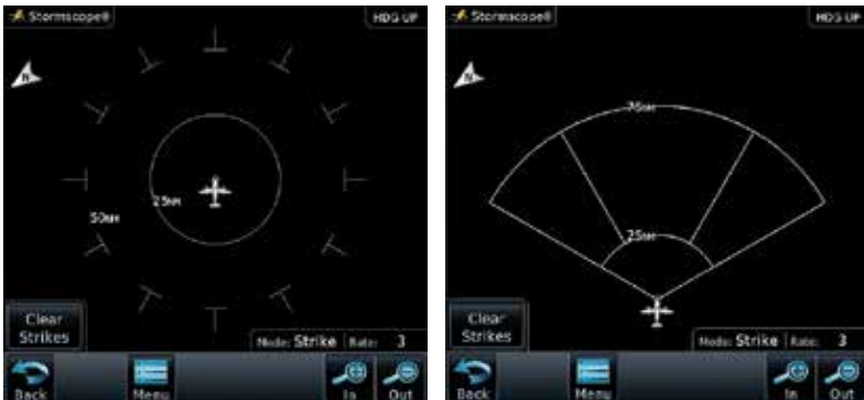
Figure 12-47 StormScope 360° and Arc Display Views
