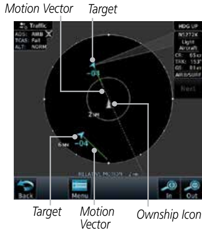
Figure 10-16 Comparison of Absolute and Relative Motion Vectors With a Two Targets
