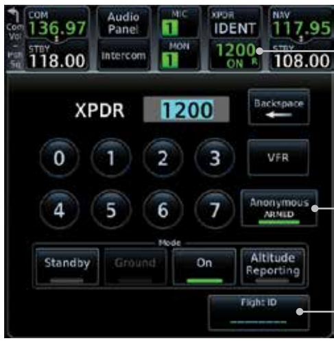
Figure 2-11 ADS-B/Transponder Control Panel
