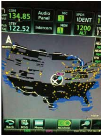
Figure 12-96 Example of Areas Where FIS-B Reception Is Unavailable Continental US NEXRAD (CONUS)
