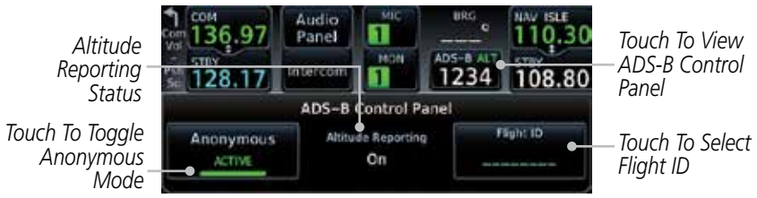
Figure 2-10 ADS-B Control Panel
