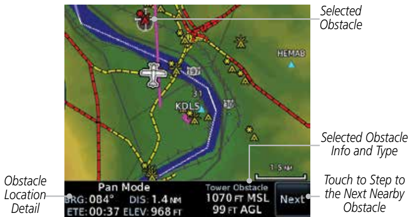
Figure 9-23 Point Obstacle Detail
