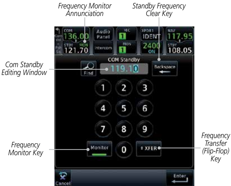
Figure 3-24 Com Frequency Monitoring
