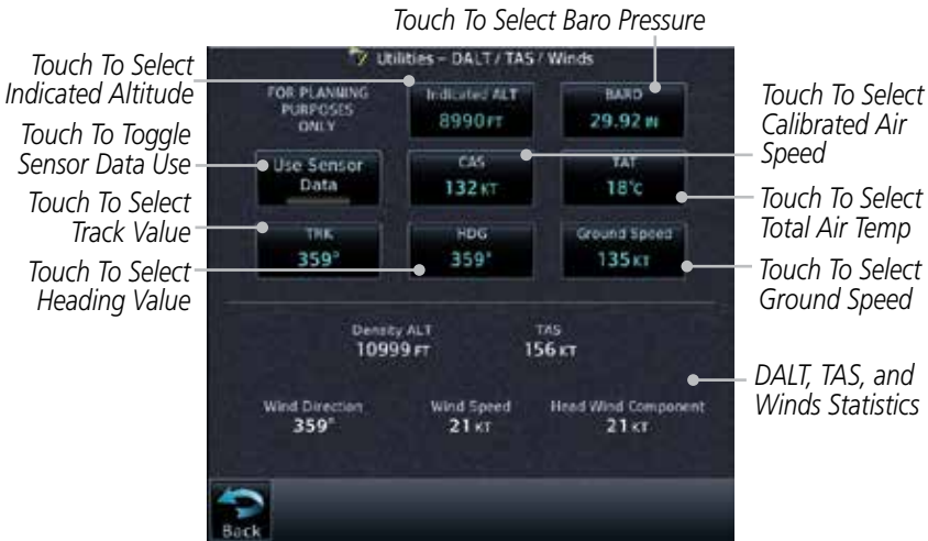
Figure 15-37 Utility DALT/TAS/Winds Page Using Manually Entered Data
